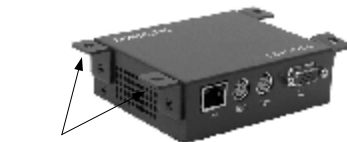
Screw L-shaped brackets to 1 or both sides of the unit
