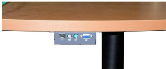
Figure 4 – IP Control Unit Connected to a Tabletop
