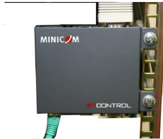
Figure 3 – IP Control Unit Connected to a Rack
